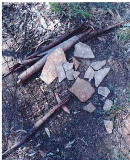
Photo 2 – Asbestos Cement Fragments at TP30
